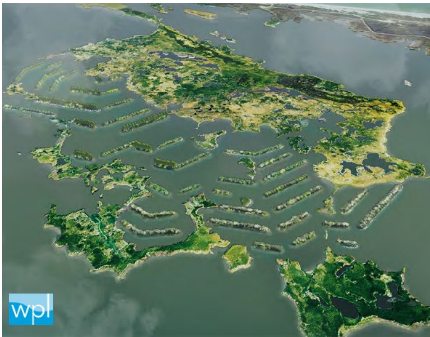
Figures 9 (above) and 10 (left): Marsh Terraces designed for land and habitat restoration and flood protection purposes in Back Bay, Virginia (City of Virginia Beach).
